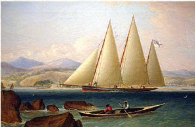
A large Bermuda sloop, built for the British Royal Navy, about 1750, with typical raked mast and fore-and-aft Bermuda Rig: the greatest invention in sailing technology after the European "Square Rigger": Dr. Edward Harris
